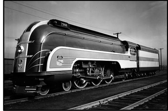
Union Pacific Streamlined 4-6-2 steam engine (photo from steamlocomotive.com)
